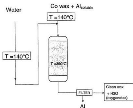
Experimental set up for removal of aluminium.
