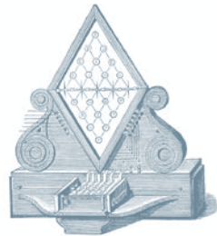
Fig. 750.—Cooke and Wheatstone's Five-Needle Telegraph.
